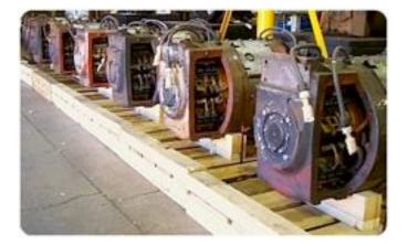
Super Lube<sup>®</sup> Silicone Dielectric and Vacuum Grease has superior vacuum capabilities for rebuilding electrical traction motors used to power passenger trains. Part of the process involves varnishing the motor components with an insulating material. The varnish must be kept from coating the commutator, bolt holes, threaded fittings, bearing shafts and electrical connections.
